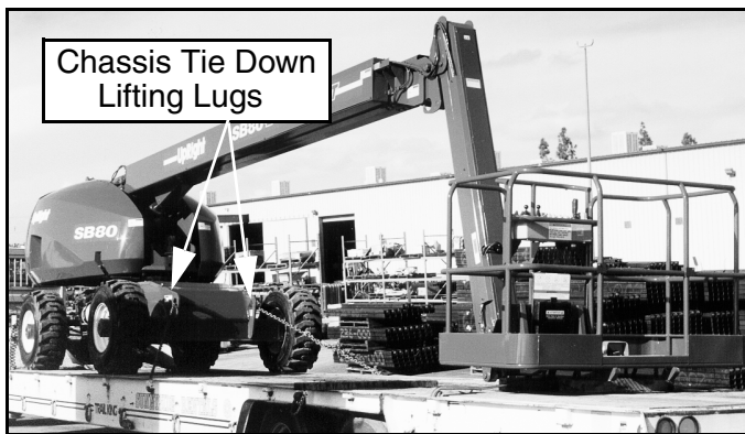
Figure 2-7: Rear chassis tie down lifting lugs
