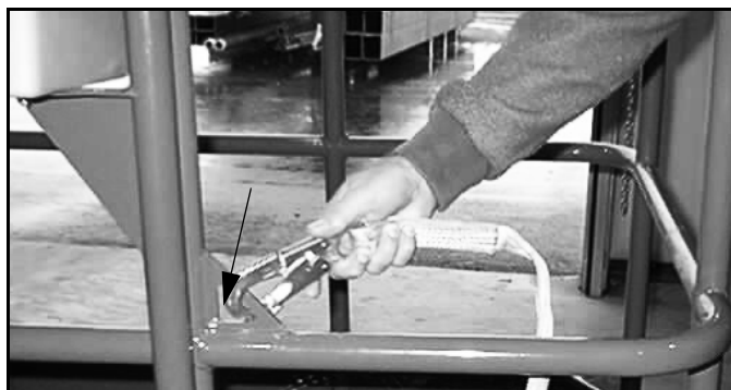
Figure 2-3: Typical Fall Restraint Anchorage Point
