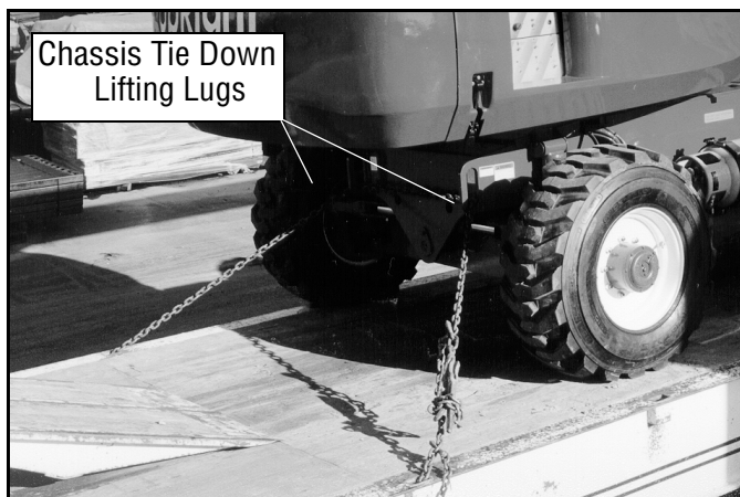
Figure 2-5: Front Chassis Tie Down Lifting Lugs
